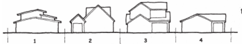
The revised design of House no. 3 became compatible with its neighbors by stepping back the second story and providing variation in the roof and building forms.
